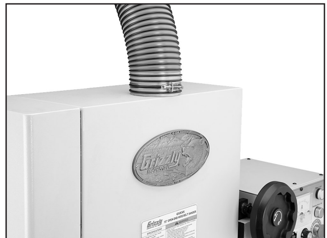
Figure 14. Dust hose attached to dust port.
